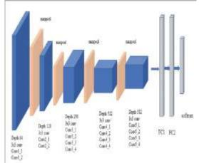
Figure 3.2: Architecture of VGG-16-CNN model
